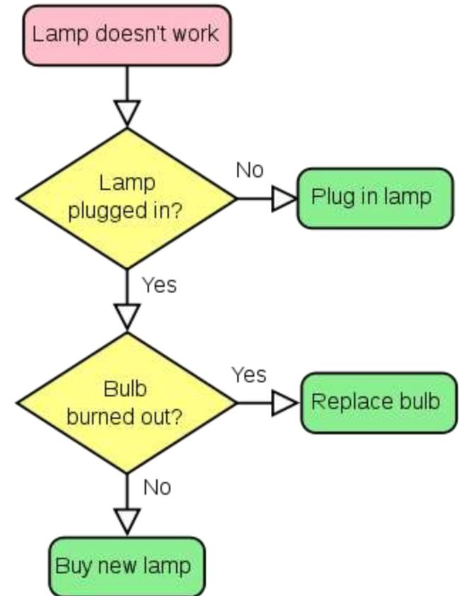
This is an algorithm that tries to figure out why the lamp doesn't turn on and tries to fix it using the steps. Flowcharts are often used to graphically represent algorithms.
